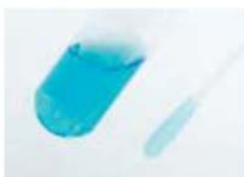
Figure 1. Flocked swab elutes specimen more efficiently.
